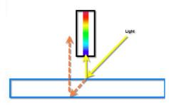
If the printed side is behind the glass, towards the diffuser, reflection measurement is not possible. The reason is, that the light is not reflected back into the optics.
