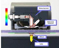
The measuring head touches the glass and is in a distance of the glass thickness to the lamp/ diffusor. In this situation, the measuring head can see also light coming from outside and therefore cause wrong readings. This error does affect only dark colors.
