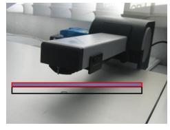
Print side behind (towards diffusor): the thicker the glass, the more light can come sideways into the measuring head causing erroneously dark patches to become lighter.
