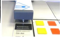
and then continue spot measurement on the patch to be measured:
